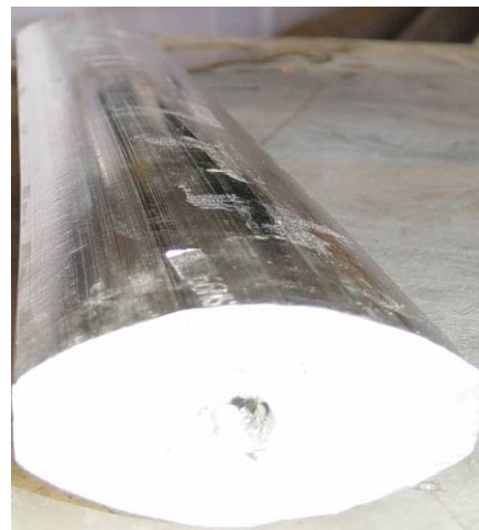
Dimension of Tin Anode 3" X 2" X 1" upto 32" Long
